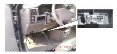
\*GM Buick GL8: the OBD plug is below the dashboard, use SMART OBDII-16 connector.
