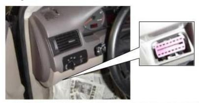
\*AUDI A6: the OBD plug is on the lower left side of the dashboard, use SMART OBDII-16 connector.
