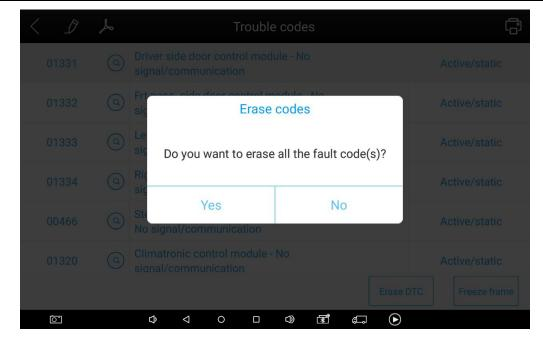
**4.5.2.** Click **YES** to confirm the operation, if the communication is normal, it will show "**Trouble Codes has been Cleared Successfully**" or "**Trouble Codes Cleared**". Generally, users will need to re-read trouble codes after clearing them to confirm that the trouble codes have been cleared.
