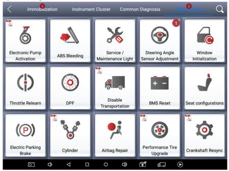
4.2. Test Functions: it can read and clear faults codes for all systems of vehicles.4.2.1. Using BMW as an example, select Common Diagnosis, then select EUROPE. Choose the BMW word. If the word is not showing on the screen, please swipe up or down to display it.
