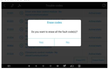
Tip: When detecting the faulty vehicle, if the display system is normal or has no fault code, it means that the relevant fault code is not stored in the ECU or some fault
